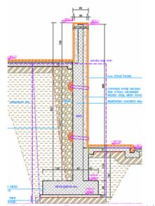
Figure 2: Retaining wall near stair No.10 original design
